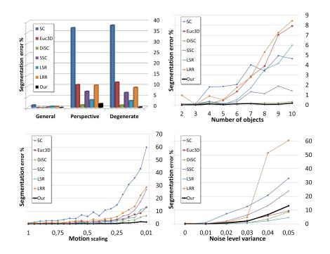
**Fig. 7.** Results from the synthetic dataset of segmentation error vs different types of motions (upper left), increasing number of objects (upper right), decreasing trajectory length (lower left) and increasing noise (lower right). Our method is displayed in bold.
