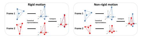
**Fig. 1.** Overview of our method. Given a set of rigid points (e.g. 4) in 2 frames, we can find a canonical representation, which allows us to compare the points between frames. For rigid motions (left example), the canonical representations will be near-identical. For non-rigid motions (right example), the canonical representations will differ considerably.
